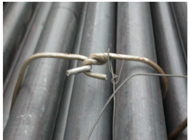
Drahtbündelung bundle with wire
