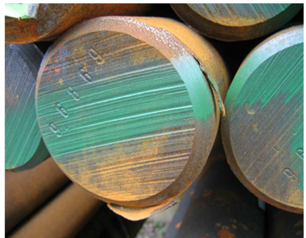
Fase am Kopfende zu groß shamfer at the end too large
