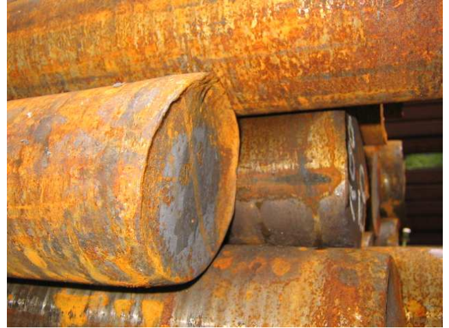
Verformte Stangenenden deformed billet / bar ends
