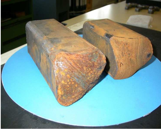
Verformte Stangenenden deformed billet / bar ends
