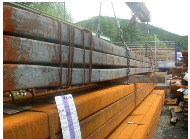
Verbogene Stangen bended billets / bars
